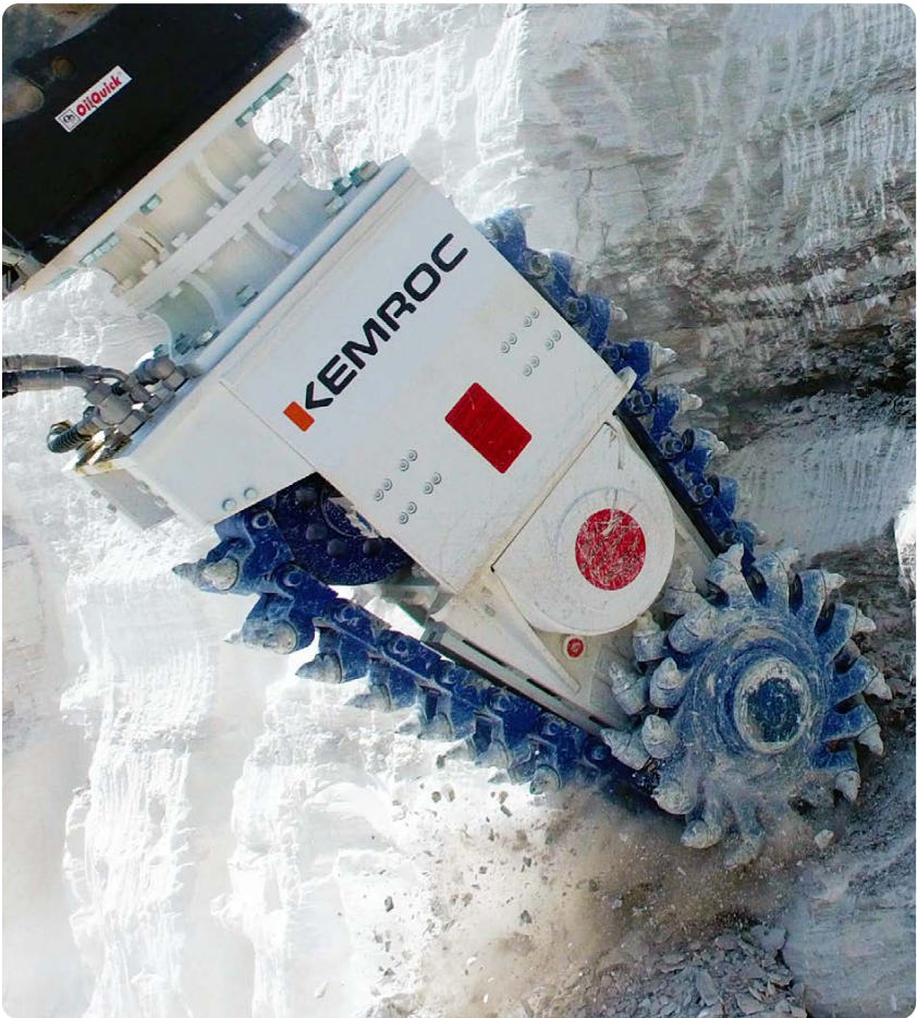
▲ Mining gypsum with an EK 100.
